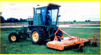
Front-Mount Mower Built From Old Deere Combine
