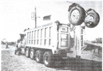
Our add-on, drop-down rear axle mounts behind big dump trucks and adds three to five tons of capacity, depending on the type of truck and number and type of axles on the truck. It provides maximum payload capacity, especially when there's no room for another axle underneath the truck. We're seeing more interest in it because new fed-
