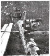
I saw logs into lumber for my own use using a Stihl 041 chain saw attached to a bracket that pulls along the top of a 2 by 4 on top of the log. A winch powered by a 1/2 hp. electric speed reducer pulls the saw slowly through the log. (Edgar Maurer, 3443 Dawley Rd., Ravenna, Ohio 44266 ph 216 296-5636)
