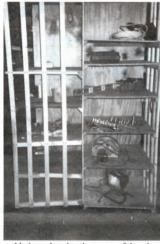
welded a pedestal to the center of the wheel and used a tapered timkin bearing for the shelves to turn on. I used some new and some used lumber to build 4 sets of 24 by
