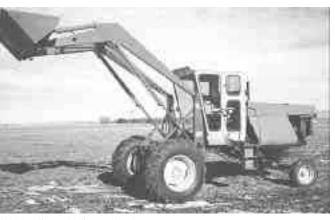
I built a self-propelled front-end loader tractor based on the one built by William Leiser who was featured in the "Best of FARM SHOW Video - Volume I." Leiser, of Grand Island, Neb., built two combine loaders, one out of a 1966 Deere 95 Hydro and another out of a 1976 International 715 Hydro. He fitted both with Deere 158 loaders.
