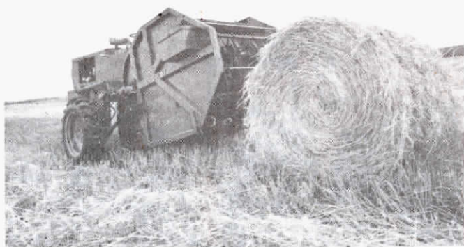
Hydrostatically-driven Swath Roller mounts on front of self-propelled swather base unit (minus swather header). Swath is rolled up on the ground to form bale.
