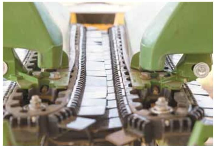
The 360 Yield Saver uses a series of flat, pliable paddles that intersect to create a continuous and flexible platform. Stalks are pulled down through the deck plates and snapping rolls without letting kernels pass through.
