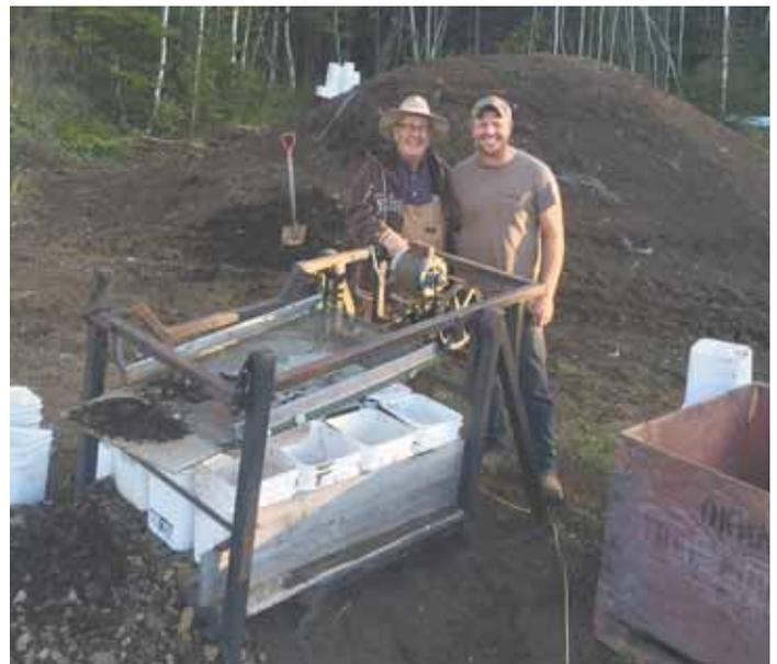
Joe Cogswell's dirt shaker breaks up clumps of black dirt into small particles, and also mixes the dirt with worm castings produced in Cogswell's vermicompost operation.
