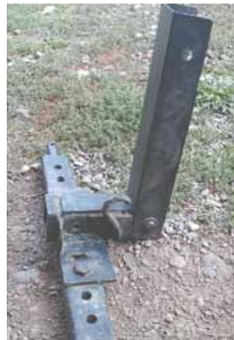
Justin Draney uses this receiver hitch on his Allis Chalmers WD tractor. It bolts to the tractor's drawbar and 3-pt. top link.
