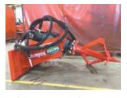
Skid loader-mounted Stumpex cutter bit uses weight and high torque while operating at a low 7 to 17 rpm's. The slow speed reduces flying debris.
