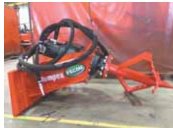
Skid loader-mounted Stumpex cutter bit uses weight and high torque while operating at a low 7 to 17 rpm's. The slow speed reduces flying debris.
