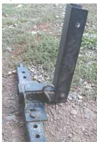
Justin Draney uses this receiver hitch on his Allis Chalmers WD tractor. It bolts to the tractor's drawbar and 3-pt. top link.
