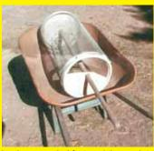
hardware mesh. I fastened the mesh to both lids, then cut away part of one lid to make an opening for filling it up. I drilled a hole through both lids that's big enough for a round wood handle and then ran the handle all the way through, wedging it in tight.
