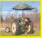
I mounted a 6-ft. wide patio table umbrella on my Deere 50 tractor. I attached a 1 1/4-in. dia. pipe to the tractor drawbar for it to fit into and also Velcroed it to the tractor seat. The umbrella happened to be green like the tractor. It works great and really makes a difference on hot, sunny days.
