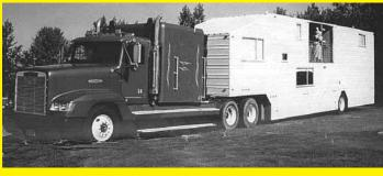
Nearly 11 years ago, FARM SHOW ran a story on a 46-ft. long, 2-story camper I built that had a porch and even a garage. The open air 8 by 9-ft. porch was on the top level while the 12-ft. airtight garage in back could be used to carry a smaller car.
