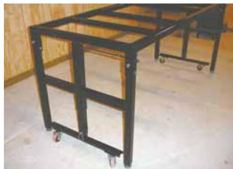
Modified trailer tongue jacks at either end of workbench - operated by a cordless drill fitted with a socket adapter - are used to lower bench wheels onto floor.
