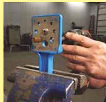
Thread Wizard uses a wire wheel that protrudes into size-specific holes surrounding the wheel. Rotating a bolt inside a hole removes all dirt and surface rust.
