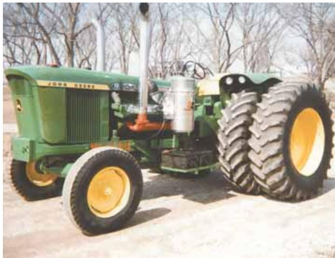
David Will replaced the locked-up engine on his Deere 5020 tractor with a Detroit V-12 diesel engine with about 450 hp. "I use it to pull a 30-ft. field cultivator. It's really loud," says Will.
