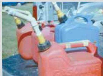
cutting off the flex part of the old spout. I left the base of each spout so I could fit a piece of pipe into it. I cut about 3/8-in. off the end of a pipe fitting and slipped it over a piece of 3/4-in. pipe so I could slip it into the old nozzle stub. I glue that into the old nozzle. Then add a 45 degree "L" and another short pipe and a pipe cap on the end. You can glue the pipe together because the entire assembly will still pivot on the cap. This cheap do-it-yourself nozzle doesn't leak."
