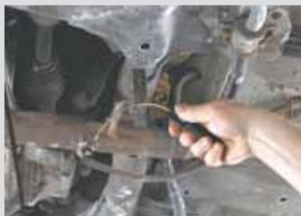
**George Burkhardt, San Antonio, Texas:** "George came up with the Drain Plug Pro to eliminate the need to touch hot drain plugs or get hot oil on hands when changing oil. You simply loosen the plug and magnetically attach the one-size-fits-all head of the tool.
