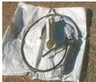
**Tom Lass carries his 5-ft. long grease gun hose extension in a homemade holster, made from 3-in. dia. pvc pipe, that hangs from his belt.**
