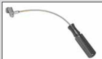
Then turn to remove the plug. No more dropping a plug into hot oil and it keeps splashing to a minimum. He came up with the tool after many years of changing oil on all kinds of equipment and getting hot oil splashed into his eyes, on the floor, and so on. The tool is sold at Amazon.com and is also available from Snap-on Tools, Matco
