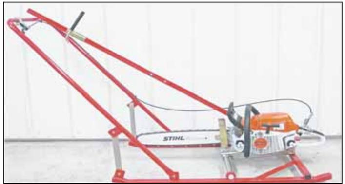
New ice cutter comes with adjustable width runners and clamps to hold a chainsaw in place. Chainsaw is operated by a remote throttle.
