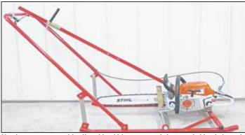
New ice cutter comes with adjustable width runners and clamps to hold a chainsaw in place. Chainsaw is operated by a remote throttle.
