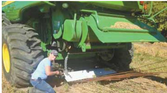
Buncher on back of combine is used to collect straw and chaff, which falls on buncher's steel fingers. As pile builds, buncher's back end gradually tilts to the ground.
