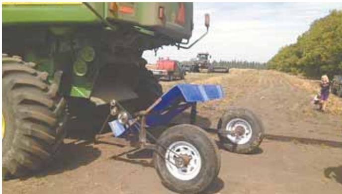
Stubble sticking up through fingers pulls the pile of bunched chaff and straw off. But that didn't work with peas, so instead Kenyon uses a ground-driven, 2-wheeled cart.
