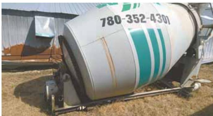
Entrance to mixing barrel is easy to load with any carcass the size of a large ewe or smaller. Winchell adds sawdust or straw and moisture.
