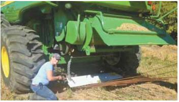
Buncher on back of combine is used to collect straw and chaff, which falls on buncher's steel fingers. As pile builds, buncher's back end gradually tilts to the ground.
