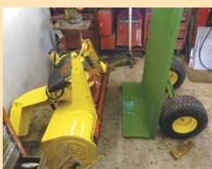
Wagon can be tipped vertically like a 2-wheel dolly to pick something up, then dropped down horizontally and hitched to the front axle for moving around.
