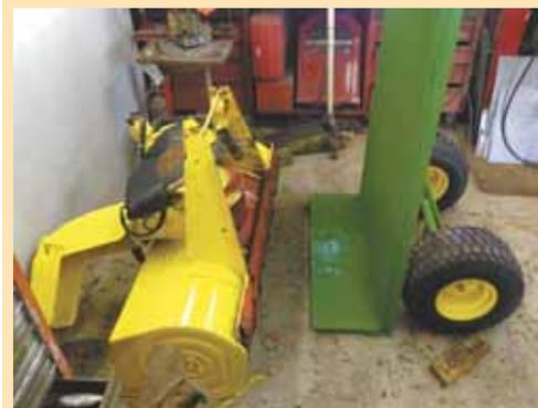
Wagon can be tipped vertically like a 2-wheel dolly to pick something up, then dropped down horizontally and hitched to the front axle for moving around.
