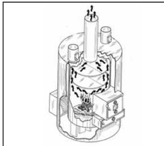
Stove design burns efficiently thanks to its round design, especially the round cast iron baffle that's parallel to the fire grate. "Baffle holds back heat and smoke, increasing the pressure, which means higher efficiency for combustion."
