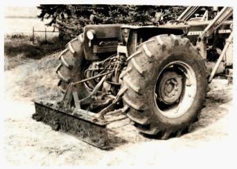
I-Beam Barnyard Scraper — Robert Sperfslage, Greeley, Iowa, made a 3-pt. scraper blade out of an old metal I-beam. He simply mounted a piece of heavy steel I-beam, about the right width to fit behind his small Massey Ferguson tractor, on a 3-pt. linkage. He says it works great for scraping alleys in barns.
