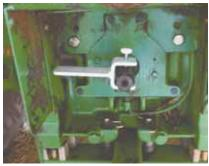
Y-shaped wrench turns pto shaft with enough leverage to easily line it up to implement.
