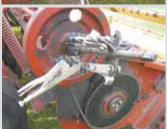
slightly. The jaws will now tighten around the shaft behind the bearing. You can move the jaws around the shaft until they're equally spaced.
