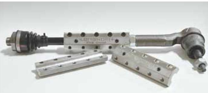
**Bolt-on sleeves from Longhorn Fab Shop make it easy to toughen up tie rods on the GM Duramax pickup.**
