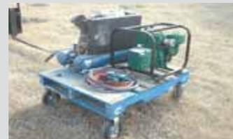
**Darry Markle, Claresholm, Alberta:** "Mounting four 8-in. pneumatic wheels on a pallet makes it easy to move my gas-powered compressor and generator around my shop. I mounted a pair of caster wheels on one side and fixed wheels on the other.
