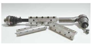
Bolt-on sleeves from Longhorn Fab Shop make it easy to toughen up tie rods on the GM Duramax pickup.
