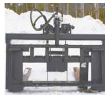
Grapple opens up to 6 ft. vertically to grab a lot of material at a time. Front and rear cylinder pivot points are adjustable for height and pull.
