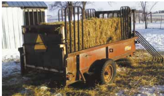
An old manure spreader works great as a big square bale feeder for Richard Haskin. He added a homemade gate across the back and used bleacher components to make sides.
