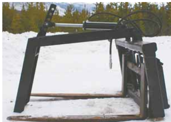
John Betka started with a set of forks to build his own quick-tach grapple for only $250.
