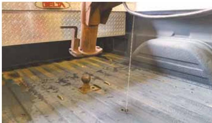
**"Backup guide" keeps gooseneck hitch from tearing up pickup's tailgate whenever Bunce drives out from under the trailer after unhooking it.**
