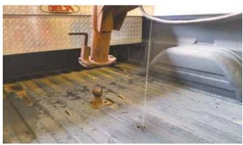
"Backup guide" keeps gooseneck hitch from tearing up pickup's tailgate whenever Bunce drives out from under the trailer after unhooking it.
