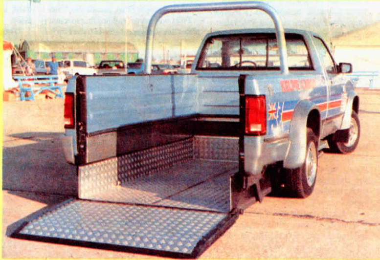
The rear axle and differential have both been eliminated to allow the bed of the pickup to move down flush with the ground. The pickup has 90 cu. ft. of capacity and a payload capacity of 1,800 lbs.
