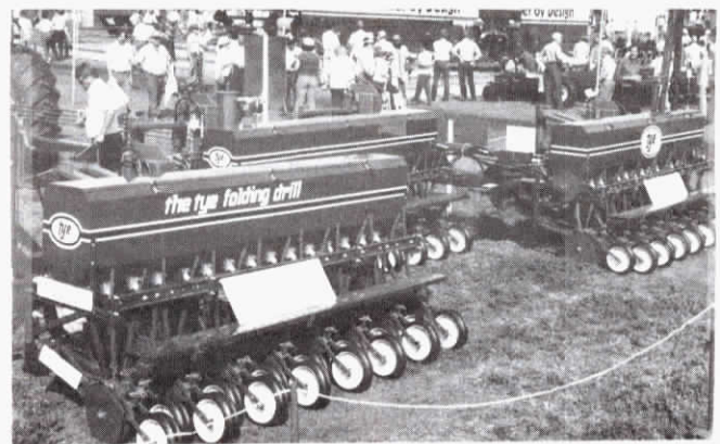
The new-type 40-ft. drill folds up to 12½ ft. for transport.
