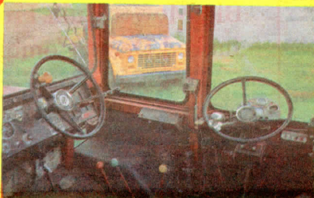
Canadian farmer mounted a second steering wheel on the side of his tractor cab and modified the seat so it swivels toward either steering wheel. Lets him do field work without having to look back over his shoulder... see p. 3. "Side Steer" Tractor Has Two Steering Wheels
