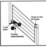
I built this "latchless" gate years ago and it works perfectly. All you do is push it open and push it shut. Nothing to fasten. It's ideal for a big board gate 12 to 14 ft. long. When closed, the gate is held by a notched 2 by 6 in. board that's sloped toward the ground. When open, the gate rides on the 2 wheels. When you push the gate shut, it slides up the slope of the 2 by 6 and drops into the notch. When you push on the gate to open it, the leading wheel, which is 18 in. out from the
