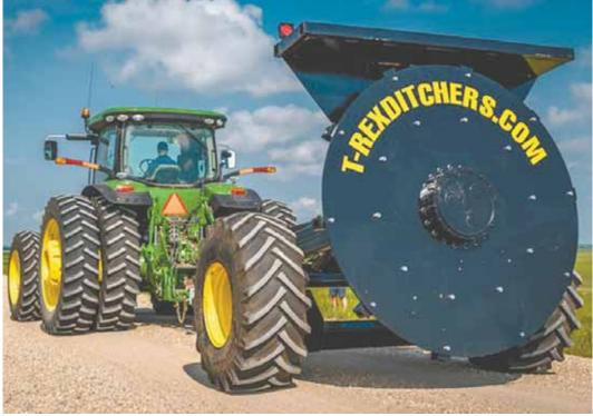
With its 8-ft. spinning wheel, the T-Rex Rotary Ditcher moves up to 10 times more dirt than pull-type scrapers, backhoes and dozers. And, it throws dirt evenly over a 300-ft. distance without leaving big piles.
