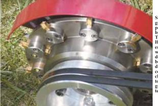
Stump grinder is powered by a Tecumseh HM80 engine, which double beltdrives the centrifugal clutch to the grinder's teeth.
