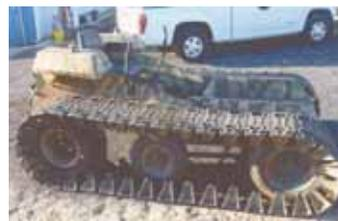
James Bassett converted a Yazoo zero-turn mower into this camouflaged marsh buggy, which rides on tracks that go around 3 sets of wheels and axles. Photo below shows original mower.
