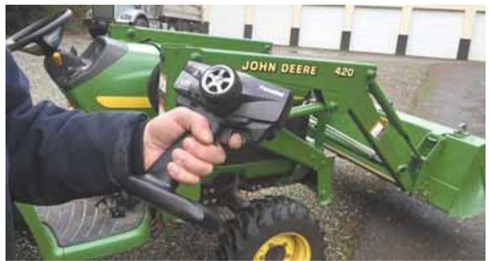
Brian Laine used mostly off-the-shelf parts to convert his Deere 4210 to a remote-controlled tractor. A standard RC controller is used to operate the tractor.
