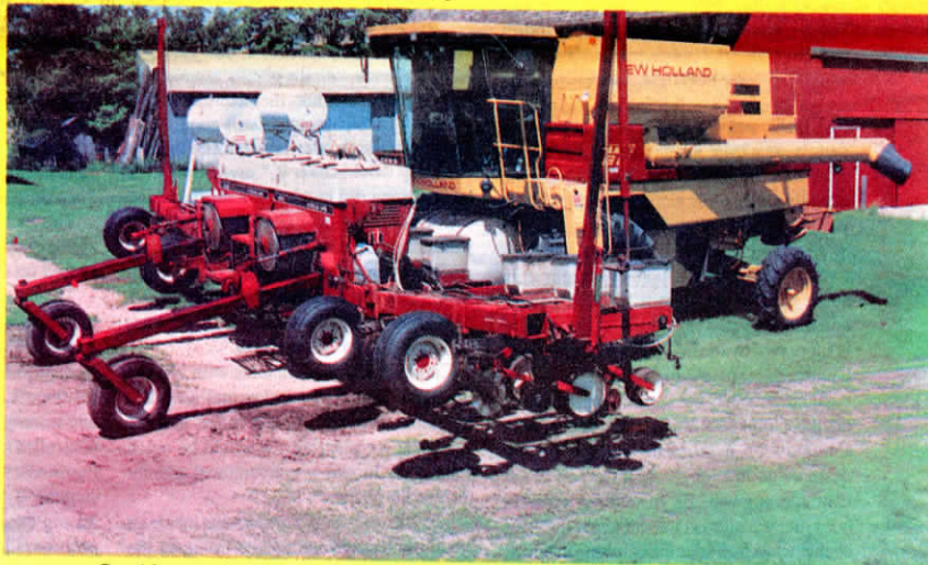
Combine carries front-mounted planter with no problems, says Carney. Two lift assist wheels were added to front of planter, which attaches to a frame bolted directly to combine axle - not the feederhouse. "It's easy to maneuver in the field and visibility is great," he notes.
