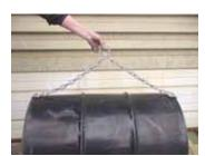
Horizontal drum lifter consists of a 4-ft. long chain with curved metal brackets welded to each end.
