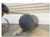
Operator grabs onto drum laying horizontally and stands it up by hand.
