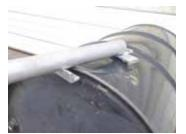
Drum tipper works like a big prybar and consists of a long pipe with 2 short angle irons spaced about 10 in. apart.
