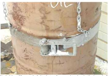
Vertical drum lifter uses the fuel tank strap from a semi-truck and a "load-securing' ratchet strap to lift drum vertically.
