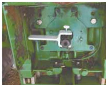
Y-shaped wrench turns pto shaft with enough leverage to easily line it up to implement.
