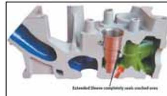
The sleeve is sealed into the head with a retaining compound and never needs replacing. Wagner says anyone comfortable with changing a 6.0 injector should be able to effectively complete the repair. He’s also proud to say the kit was selected as one of the 20 most innovative new products in the automotive industry for 2015 by Motor Magazine.
