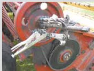
slightly. The jaws will now tighten around the shaft behind the bearing. You can move the jaws around the shaft until they’re equally spaced.
