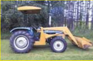
Here's a photo of my Long tractor equipped with a canopy I made using the top part of an old Allis Chalmers Roto Baler. I painted the canopy yellow to match the tractor's front-end loader. The Roto Baler was popular during the late 1940's and 1950's. It made small round bales that were only 10 to 12 in. in dia. and was the beginning of the round bale era. You can still find a lot of these balers sitting around on farms. (Duane Myklejord, 34683 350<sup>th</sup> Ave. S.E., Fosston, Minn. 56542)
