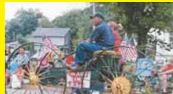
wheels are off a hay rake, with the rear wheels chain-driven off a 5 hp engine and the 3-speed transmission from a 1937 Chrysler. It'll climb a pretty steep hill.
