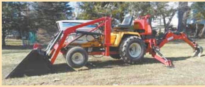
"It amazes me every time I use it," says Ken Esposito about the loader/backhoe he built out of a Cub Cadet garden tractor. "I can pick up 1,000 lbs. with the bucket and use forks to handle pallets."
