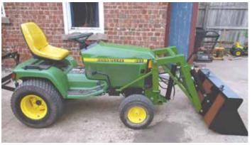
Steve Nichols built this "new and improved" mini loader that's designed to fit Deere's 425, 445 and 455 garden tractors.
