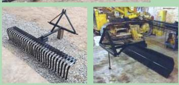
Ranette builds light to medium duty rakes as well as heavy duty models. His back blades come with 6 different angle settings and 360 degree rotation
