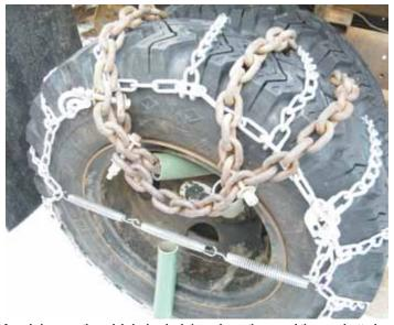
Log chain wraps through holes in wheel rim and over tire several times, and attaches together with double-nutted nuts. Short lengths of plastic hose protect wheel rim. Log Chain Used To Get "Unstuck"
