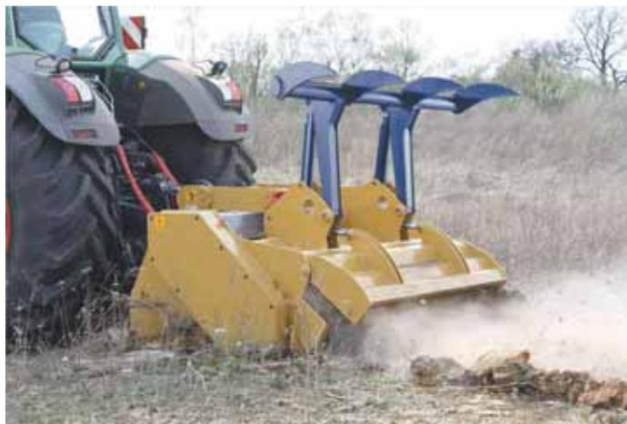
RotoCrusher’s high and low ratio gearboxes can be easily swapped to change rotor speeds, depending on whether you want to crush stones and stumps or mulch wood and small trees.
