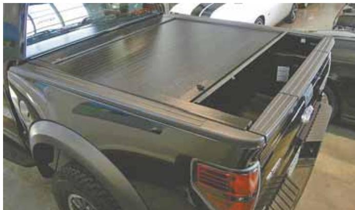
Remote-controlled pickup cover opens or closes in 30 seconds and can be locked in place anywhere along the track.
