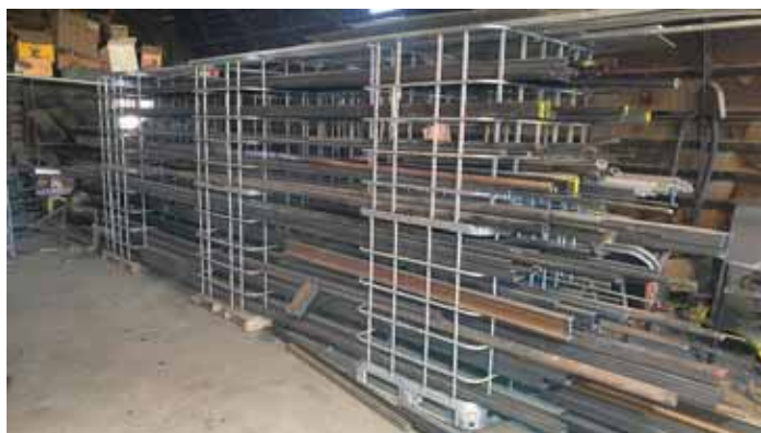
David Lehman used the metal cages on chemical shuttles to build this 24-ft. long storage rack. It consists of 3 sets of double-stacked shuttle cages spaced 4 ft. apart.
