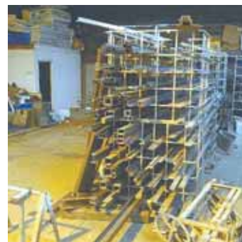
Cages have matching holes so long steel pieces will go all the way through them.
