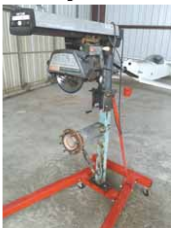
Brian Lazenby couldn't find a tire truing machine so he built his own out of an old radial arm saw and an engine hoist.
