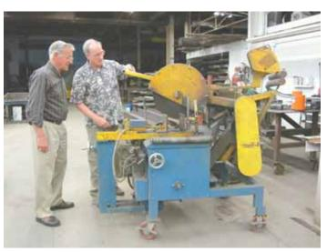
Chop saw's 10 hp. motor and 3-phase, 600-volt electrical box mount on a sturdy 1/4-in. thick steel frame.
