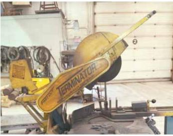
Terminator 20-in. abrasive chop saw cuts steel up to 4 in. thick.
