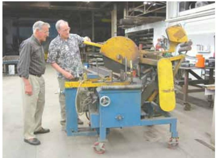
Chop saw's 10 hp. motor and 3-phase, 600-volt electrical box mount on a sturdy 1/4-in. thick steel frame.
