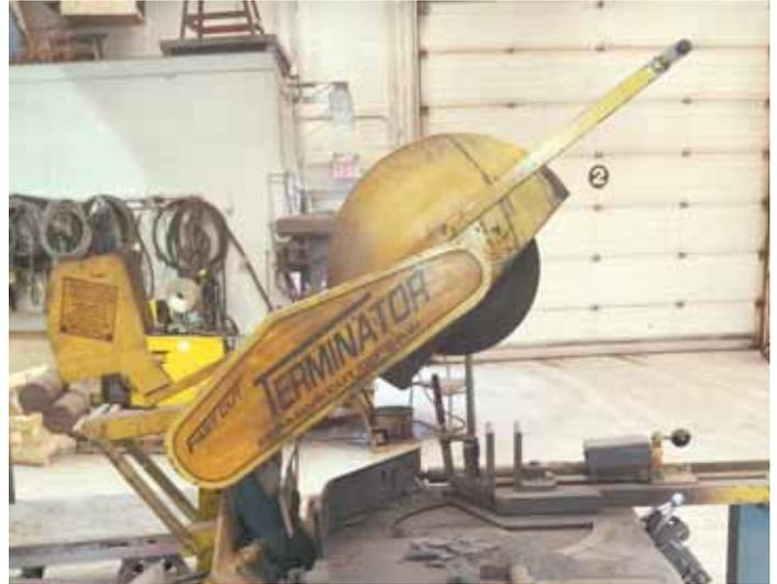
Terminator 20-in. abrasive chop saw cuts steel up to 4 in. thick.
