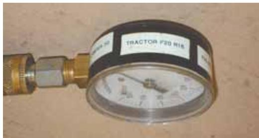
Labels attached to tire pressure gauge show the pressure needed on all of Campoli's vehicles.
