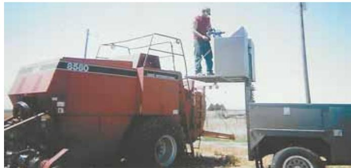
Portable workbench mounted on back of Schoenenberger's 2-ton service truck lifts up to 9 ft. in the air.
