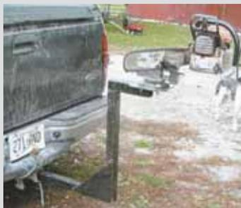
It consists of 2 pieces of telescoping tubing that slips into any standard 2-in. receiver hitch, allowing you to take the vise with you anywhere.
