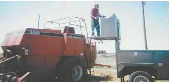
Portable workbench mounted on back of Schoenenberger's 2-ton service truck lifts up to 9 ft. in the air.
