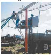
Forklift mast is used to lift a workbench. Fold-down platform provides a place to stand
